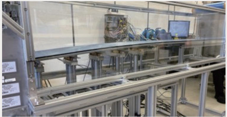
Figure1 : Photo of the experimental apparatus. The height of the basal plate is changeable in response to rising and lowering of the electronic cylinders.
