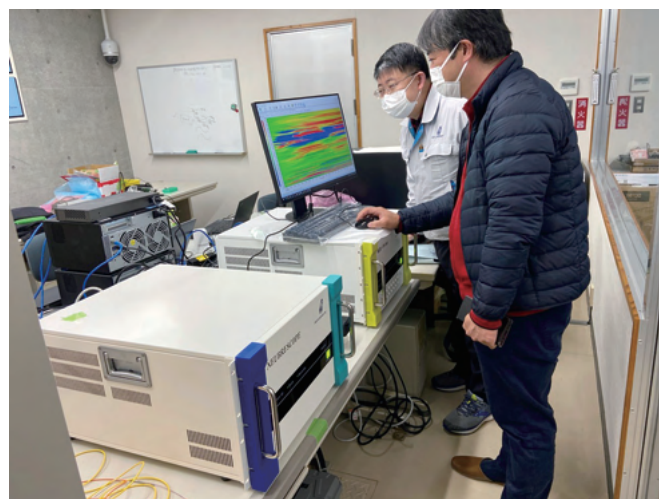
Figure 1: Left) Off-Muroto submarine fiber optic cable shore station; Right) TW-COTDR fiber optic sensing observations performed at the shore station.
